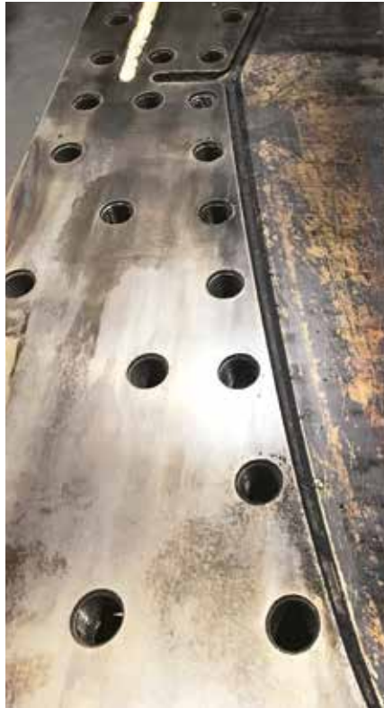
Before – after; professional die body cleaning carried out by Oerlikon Neumag restores items virtually to their original state.
